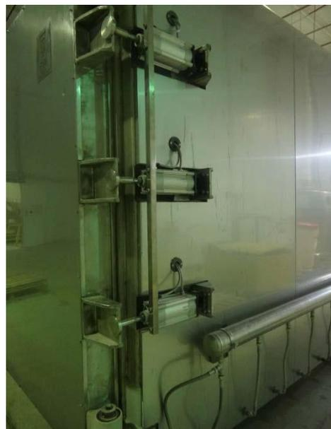
Example Figure of Pneumatic Door Closing
